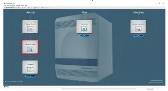
2.2 Click "Plate setup" and select "FAM" for Target1, 'TexasRed" for Target2, "VIC" for Target3, "Cy5" for Target4, and "TAMRA" for Target 5 in "Define Targets and Samples"
